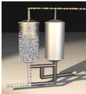
This air separation process is reliable and virtually maintenance-free. The molecular sieve will last indefinitely, as long as it does not become contaminated with water or oil vapors. This is why regular filter element replacement is crucial to trouble-free operation. The filter elements are inexpensive and require semi-annual maintenance.
