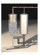
This air separation process is reliable and virtually maintenance-free. The molecular sieve will last indefinitely, as long as it does not become contaminated with water or oil vapors. This is why regular filter element replacement is crucial to trouble-free operation. The filter elements are inexpensive and require semi-annual maintenance.
